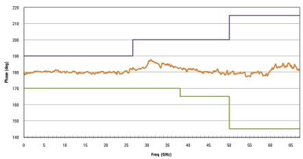
Figure 5. U9391G Comb Generator Phase at 10 MHz PRF
