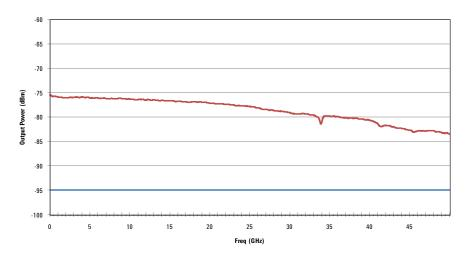
Figure 7. U9391F Comb Generator Output Power at 10 MHz PRF
