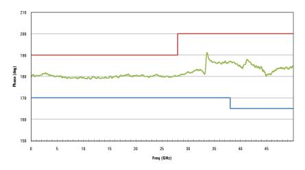
Figure 4. U9391F Comb Generator Phase at 10 MHz PRF
