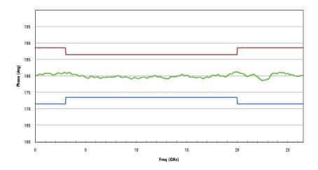
Figure 3. U9391C Comb Generator Phase at 10 MHz PRF
